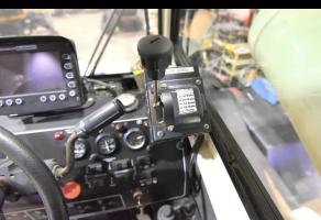
Mitchell's mobile railcar mover system for RT Cranes consists of front and rear railcar couplers and train air brake system. This dual-purpose configuration is ideal for railroad car shops used for both crane lifting operations and railcar moving. The crane functions like locomotive to move railcars without the high expense of a locomotive. The train air brake system is controlled by a cab installed stepped brake controller that progressively slows the train just like a locomotive control.
